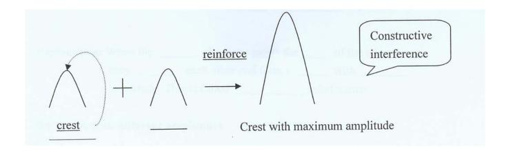
Explanation: When the <u>crest</u> of a wave <u>meets</u> the <u>crest</u> of the other wave, they <u>reinforce</u> each other and form a <u>crest</u> with <u>maximum</u> amplitude. This is called <u>constructive interference</u>.
