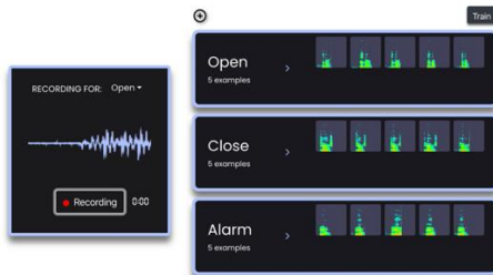
Figure 2. The label view allows users to add custom labels and record corresponding audio clips. Audio clips are up-sampled and converted to spectrograms in the browser.
